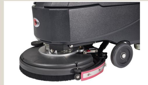
Place the brush or the pad-holder under the deck and Lower the deck or the brush/ pad holder by pressing the pedal. The squeegee is raised and lowered with the deck.
