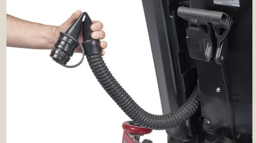
**Daily:** Empty the recovery tank using the recovery empty hose. Bend the soft part before removing the cap to control the flow.
