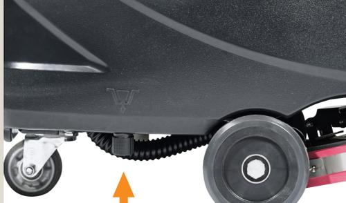
**Daily:** Empty the clean water tank using the solution tank drain knob under the machine.
