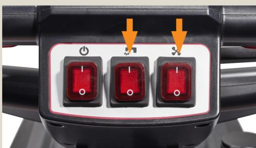
Press solution and vacuum buttons on and start cleaning by placing the hands on the safety switches.
